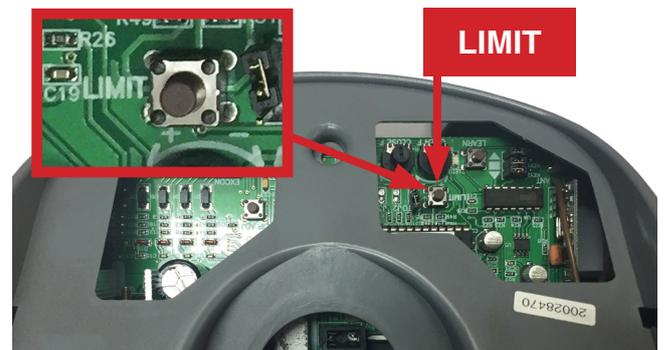
Press and hold the 'Limit' button for three seconds. The unit will beep three times to confirm the unit is in limit setting mode.
