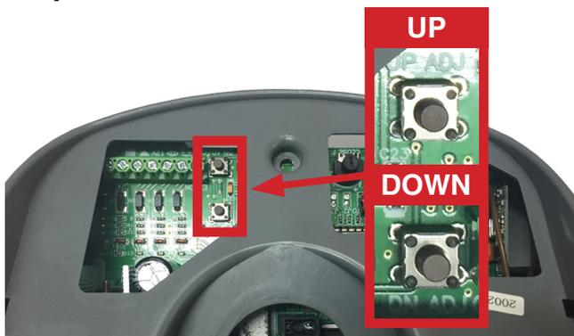
Press and hold the 'UP ADJ' button until the door travels to the desired open position. Press 'Limit' once to save this position in the units memory. Unit will beep twice to confirm. Repeating this process, press and hold the 'DN ADJ' button until the door reaches the desired close position. Press the 'Learn' button to save.
